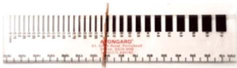
Prior to monitoring changes in the width of cracks it is necessary to measure the crack width. This is called the present condition or 'snapshot' survey. The Avongard Crack Width Gauge is specifically designed for this purpose.
